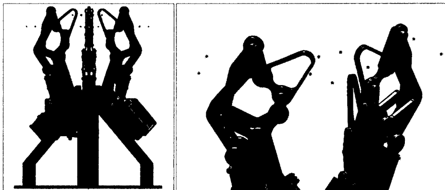
Figure 37. Concept for wrist with exterior support with attached finger linkages at a wider angle.
